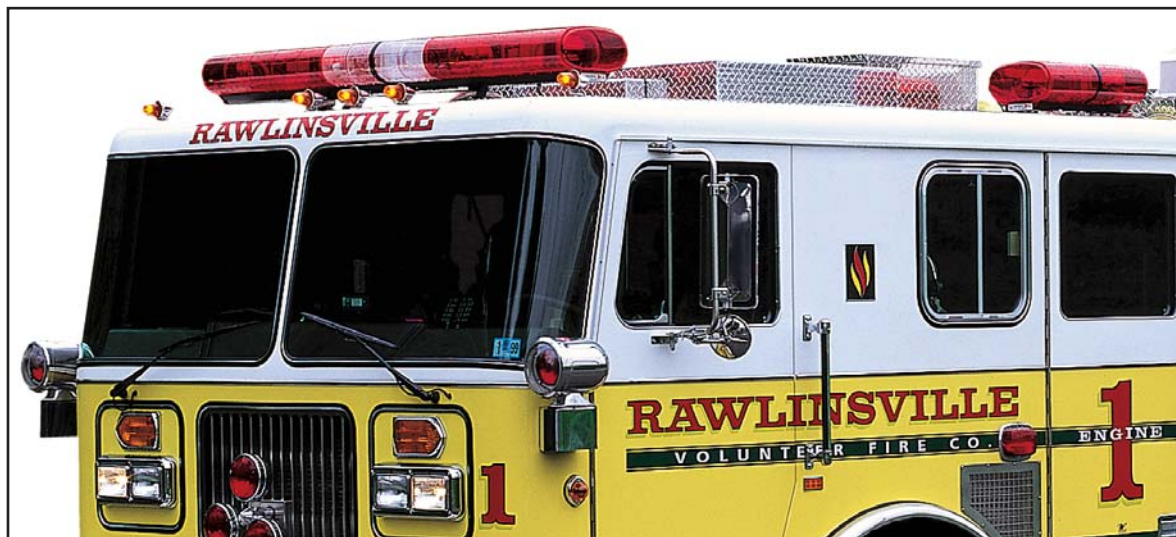
For custom fire apparatus, 22" AeroDync mini-lightbars perfectly complement full size AeroDync lightbars and provide superior warning power to the side zones of a vehicle. See bulletin #4118 for more information on AeroDync mini-lightbars.
